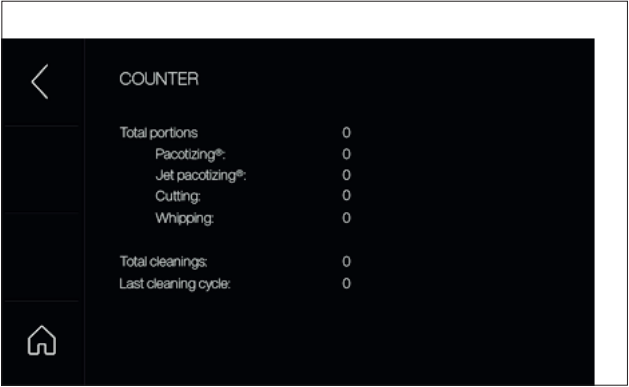
Counter: Shows the number of processed portions and cleanings.
