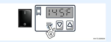
8. Allow the drawer warmer to re-stabilize and **compare** the temperature again. Tolerance at  $140^{\circ}F$  ( $60^{\circ}C$ ) is +/-  $8^{\circ}F$  (+/- $4^{\circ}C$ ). Tolerance at  $180^{\circ}F$  ( $82^{\circ}C$ ) is +/-  $10^{\circ}F$  (+/-  $6^{\circ}C$ ).
