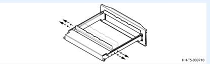
3. **Slide** the bracket to the back two (2) holes.
