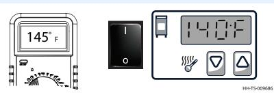
5. If the multimeter temperature and the Actual temperature don't match, **press** and **hold** the Up and down arrow buttons ② for eight (8) seconds. The control will display the previous calibration offset value or 0.
