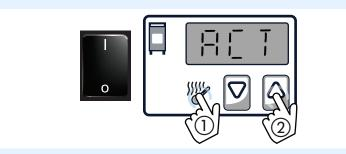
2. To return to show the Set temperature, **press** and hold the Temperature Display button (3) and the up arrow (4) for five (5) seconds. The control will display "SET" and then the Set temperature.
