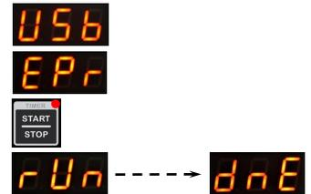
The export feature is useful for backing up the parameters in the controller, or creating a copy of the set of parameters to apply to another oven.
