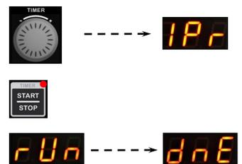
The import feature is useful for restoring a backed up set of parameters, or applying a copy of parameters from another oven.
