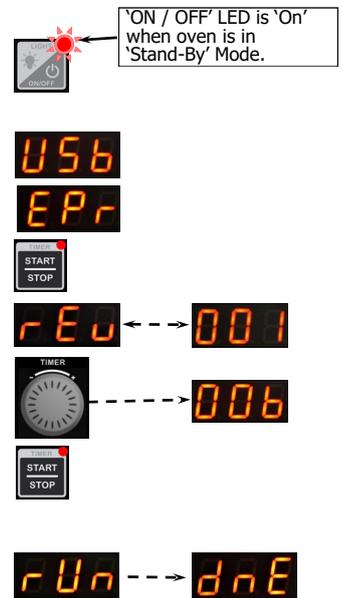
The export feature is useful for backing up the set of programs created in the controller, creating a copy of the set of programs to apply to another oven, and for editing programs externally.
