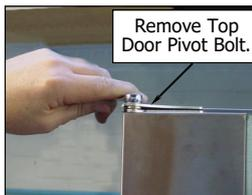
9. Remove top door hinge and fit to bottom opposite corner of door.
