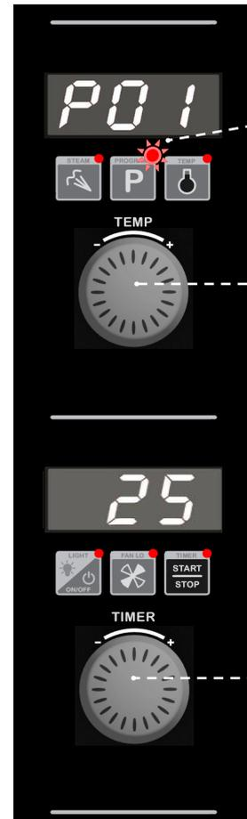
'Program' LED is 'On' when Oven is operating in Programs Mode.
