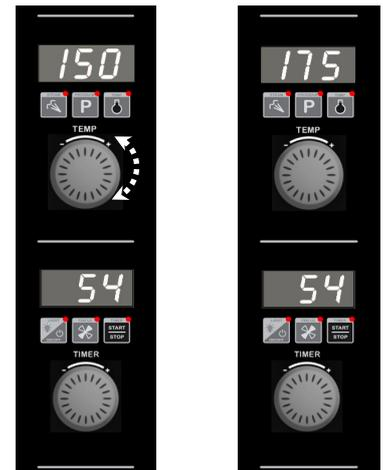
Oven Set Temperature has been increased from 150 to 175°C (325 to 350°F).
